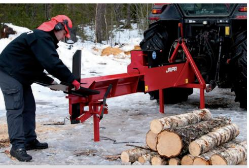
The splitting cylinder stroke of the JAPA hydraulic firewood splitter can be adjusted in accordance with the length of the log to be split.
