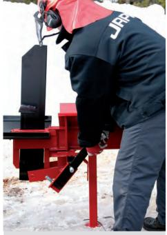
The 2/4-way splitting wedge of the JAPA 110 hydraulic firewood splitter can be adjusted with an easy-to-use lever.
